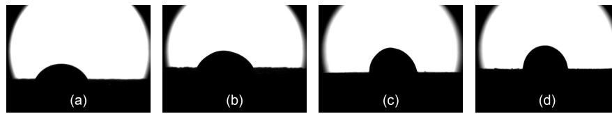
Fig. 10. Photographs of cross-linked gel droplets on sandstone at different concentrations (wt%) of SWCNTs: (a) 0.01, (b) 0.025, (c) 0.05 and (d) 0.1.
