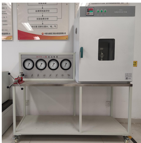
Fig. S2. Picture of the temperature–pressure reaction device.
