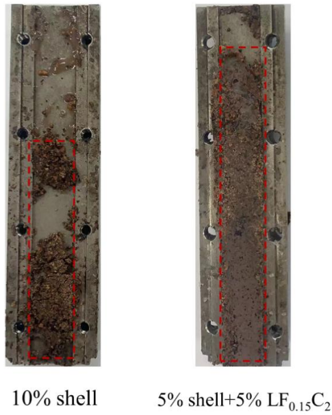
Fig. S6. The pictures of LCM in fractured metal core.
