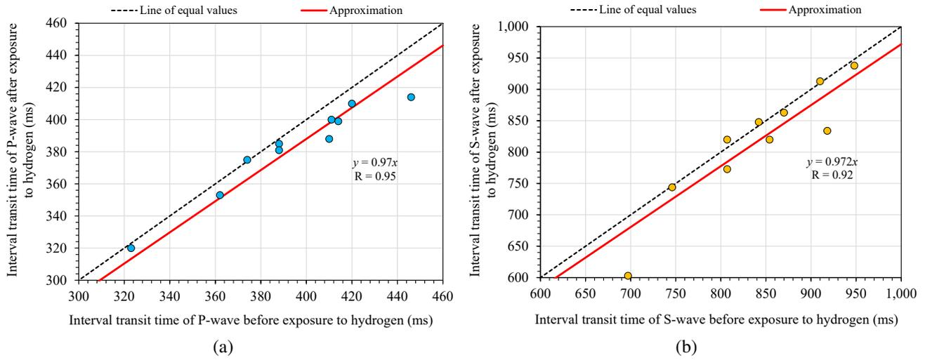
**Fig. 5.** Comparison of interval transit time values of (a) P wave and (b) S wave of core samples before and after exposure to hydrogen.
