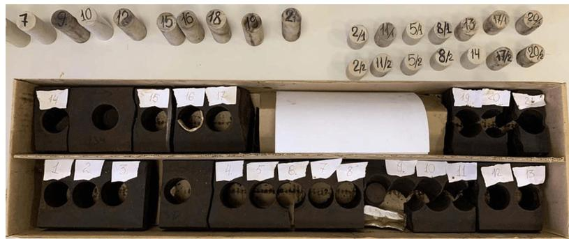
**Fig. 1.** Source core material and samples after drilling out.
