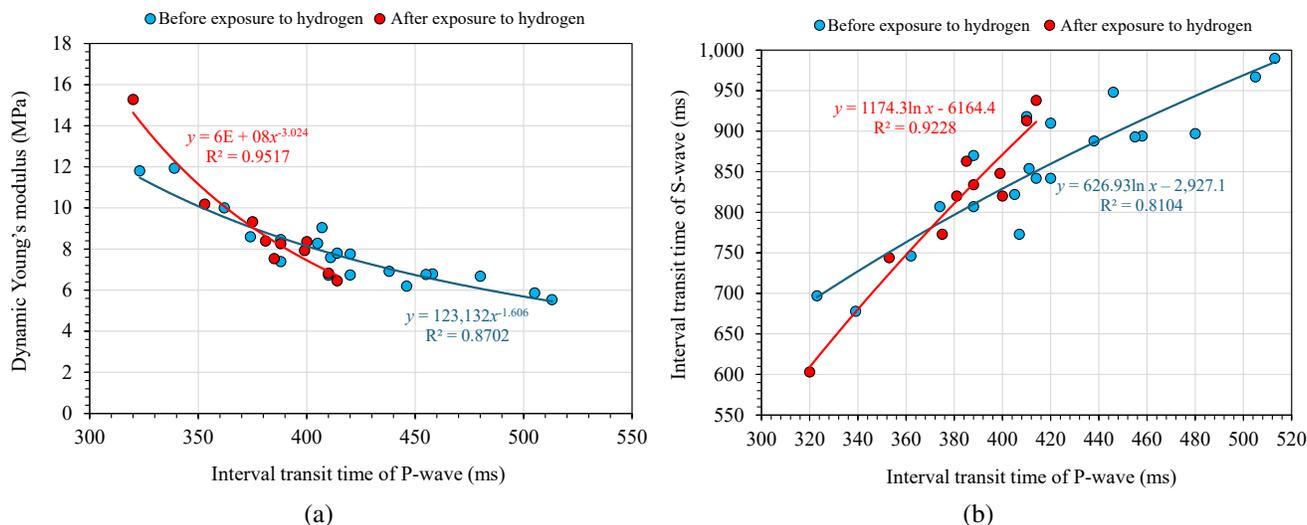
**Fig. 7.** Comparison of dependences of (a) dynamic Young's modulus and (b) interval transit time of S-wave on interval transit time of P-wave for core samples before and after exposure to hydrogen.
