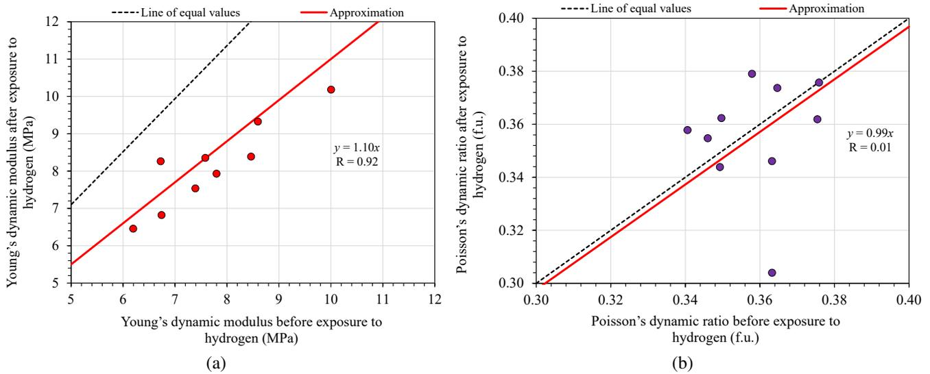
**Fig. 3.** Comparison of values of (a) dynamic Young's modulus and (b) Poisson's ratio of core samples before and after exposure to hydrogen.
