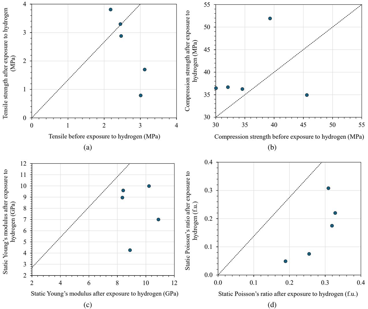
**Fig. 6.** Results of (a) determining tensile strength, (b) compression strength, (c) Young's modulus and (d) Poisson's ratio by static method for "paired" core samples (dotted line-line of equal values).
