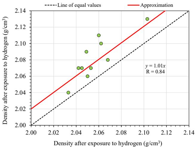
**Fig. 4.** Comparison of core samples density before and after exposure to hydrogen.
