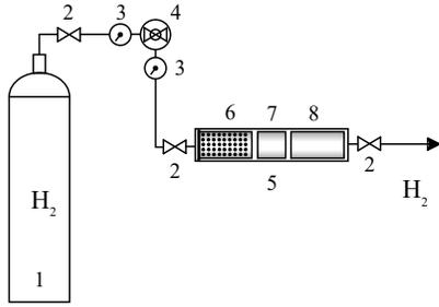
**Fig. 2.** Scheme of the unit for holding core samples exposed to hydrogen: 1-cylinder with compressed gas (hydrogen); 2-inlet and outlet valves; 3-pressure sensors; 4-pressure reducer with a valve; 5-sealed cylinder with rock samples; 6-sieve with a crushed rock; 7-standard core sample (diameter and length 3 cm); 8-longer core sample (diameter 3 cm, length 6 cm).
